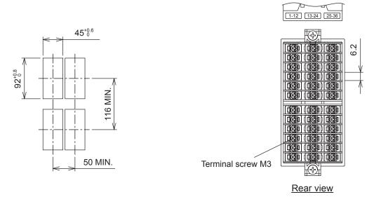
Terminal block is not attached to unused terminals (terminal 13 to 24) according to the model.
